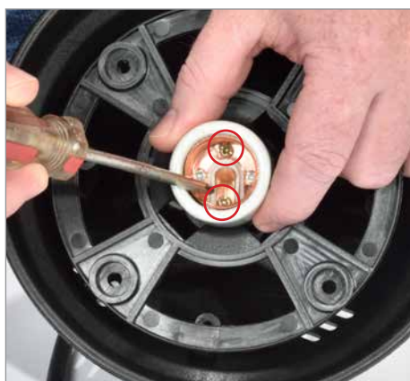
2. Remove 2 screws (circled above) holding socket to socket base.
