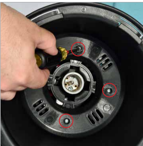
13. Place lamp dome over insert. Line up holes of dome with those of insert.
