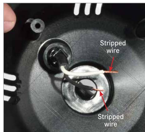
6. Use wire stripper to remove 1/2" of insulation from end of each wire.
