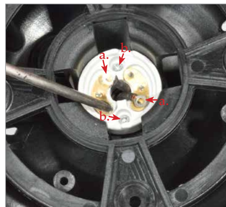
3. a. Remove screws holding ringed wires on the socket base. b. Remove screws holding socket base to lamp insert.
